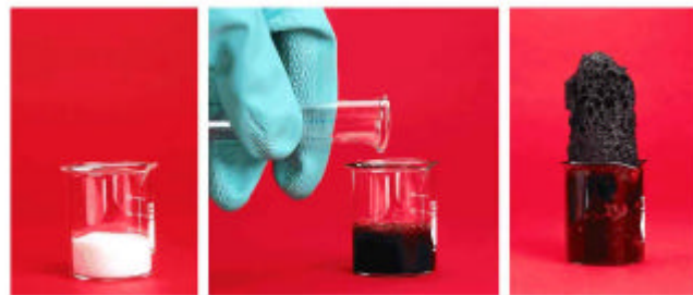
Figure 20.21: (a) A beaker of sucrose (table sugar). (b) Concentrated sulfuric acid reacts with the sucrose to produce a column of carbon (c), accompanied by an intense burnt-sugar odor.
