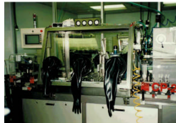
Figure 20.3: An inert-atmosphere box used when working with oxygen- or water-sensitive materials.
